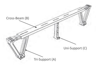
You will need 2 screws per Cross-Beam, 2 per Tri-Support and 2 per Uni-Support. We recommend  $8 \times 1\%$  wood screws. You can also use the same size screws to fix the attic boards on to the Cross-Beams.
