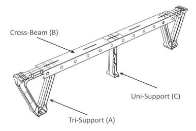
You will need 2 screws per Cross-Beam, 2 per Tri-Support and 2 per Uni-Support. We recommend 8 x  $1\frac{1}{2}$ " wood screws. You can also use the same size screws to fix the attic boards on to the Cross-Beams.
